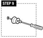
**STEP 9:** Insert long screw (i) through mounting bracket (g), then screw into plastic drywall anchor (f).
