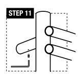
**STEP 11:** As shown in the picture, install the set screws (c) into the hole of all the tubes (a and b) using the allen wrench; fix the tube (a) onto the mounting bracket (g and h).
