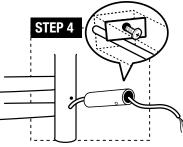
**STEP 4:** Guide the electrical cord through the electrical connection mounting tube (b) and use the long mounting screw (e) to tighten the electrical connection mounting tube to the vertical bar.
