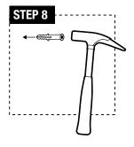
**STEP 8:** Use a hammer to knock plastic drywall anchor (f) into wall completely.
