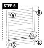
**STEP 5:** Use a tape measure to measure the distance between the center points of each wall bracket tube; record the distances between points AB, AC, CD, and BD. Mounting point C will determine electrical box location. See Electrical Assembly in following instructions.
