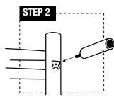
**STEP 2:** Use the short mounting screw (d) to fix the mounting tube (a) to the threaded metal pad on the vertical bar on the back of the towel warmer.
